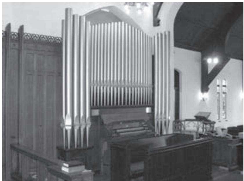
in each division to balance two colorful flutes, a Stopped Diapason and a Melodia. The organ features Diapasons at 8' and 4' pitches on the Great. Our task for the 2' was to achieve clarity without being strident. After all the pipework had undergone cleaning and regulation back to its original state, many were surprised at the return of color and speech intonations.
