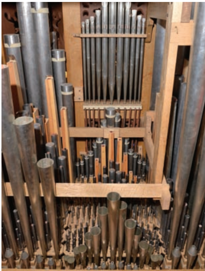
Manual pipework, including lead tubes to façade pipes
