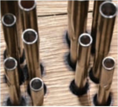
Manual Mixtur pipes with burned rack holes
