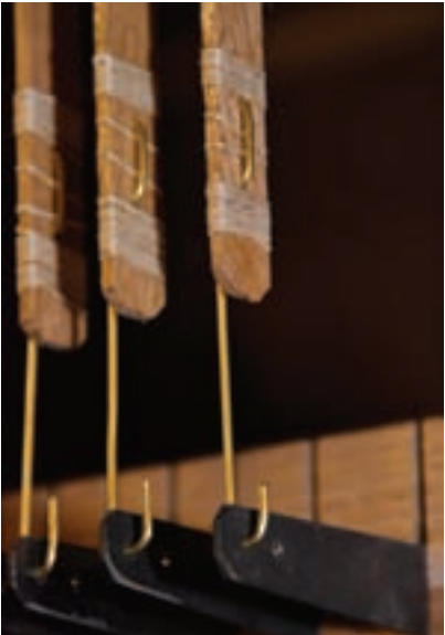
Detail view of tracker ends with hand-bent brass wires hooked into the squares
