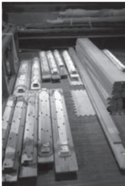
Pitman chest pouch-rails and expression shades ready for re-installation in organ
