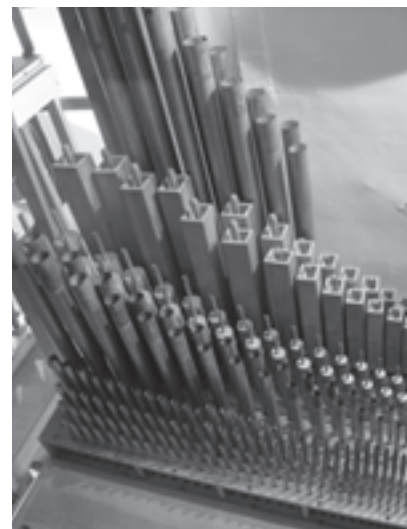
Half of the Great division, showing the 16' Contra Geigen, the 8' Holzflöte, the 4' Rohrflöte, the 2 1/2' Quint and the IV-rank Fourniture (from back to front) (photo by Andrew Forrest)
