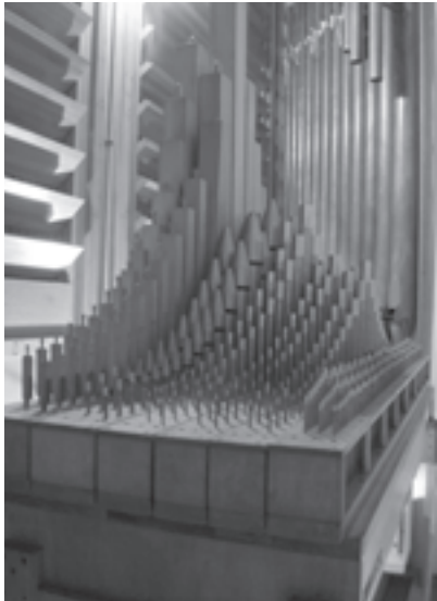
The unenclosed Positiv and 16' Flauto Dolce extension, with the Swell shutters behind (photo by Andrew Forrest)
