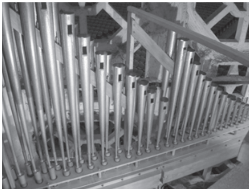
The 8'-4' Trompette en chamade rank sits immediately behind the Great / Pedal chamber grille and speaks on nearly 9' wind. (photo by Andrew Forrest)
