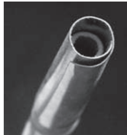
High C of a 4' flue rank showing distortion of pipe shape caused by tuning collar
