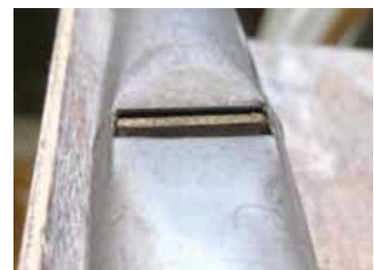
Finer nicking of the treble pipes. Note the very wide flueway. (photo courtesy: William Drake, Ltd.)
