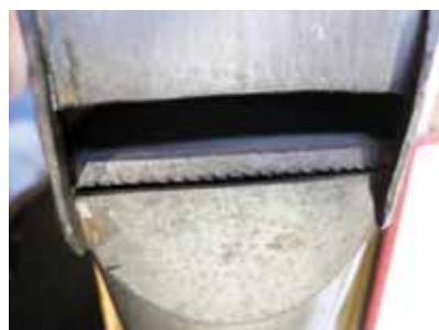
Fifteenth, GG, showing bold, slanted nicking and high languid position. Smaller pipes have finer nicks. (photo courtesy: William Drake, Ltd.)
