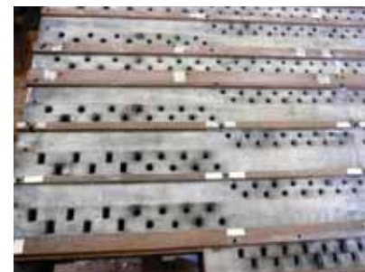
Note the parallel bass and treble slider positions on the top of the windchest with the topboards removed. (photo courtesy: William Drake, Ltd.)
