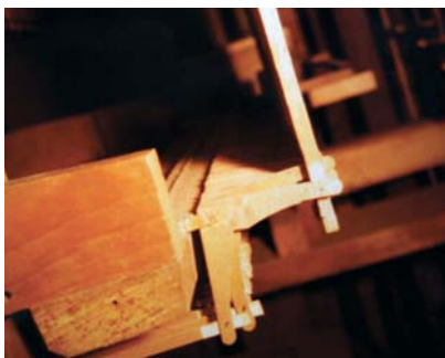
These squares are pinned directly to the trackers with no adjustment.
