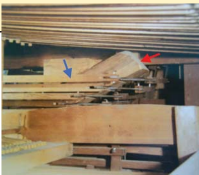
A view from the back of the console looking towards the left side with the Swell stop action. The blue arrow indicates the square shanks from the stopknobs that connect to horizontally-mounted metal squares. These squares connect to horizontal wooden shanks and another set of metal squares. The red arrow points to the diagonally-mounted beam which carries the horizontal squares; note that it has been crudely sawn off, perhaps one of the many consequences of the repositioning of the Swell windchest.
