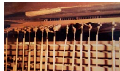
The rollerboard and trackers of the pedal coupler to the manuals; note the angled backfalls at the top connecting to the tails of the manual keyboards.
