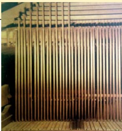
A view from the console showing the back of the Swell keys at bottom, the stickers from the Great extending upward through the Swell key tails, and the Great rollers at the top that activate the diatonic bass notes. The rollers and squares at the top right activate the Great pallets d#, c#, B, A, G, F, D#, C#. The Great pallets C, D, E, F#, G#, A#, c, d, e, f . . . g''' are activated from left to right by the fanned squares.
