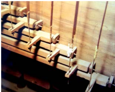
The Swell rollerboard. Note the finely-cut slots in the tops of the roller arms to minimize friction and binding. The original pencil layout marks are still visible.
