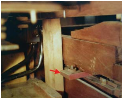
The red arrow points to the sliding board carrying the stickers in one of the couplers. Note the electric blower switch; this has been attached to the stop knob labeled "Bellows Signal."
