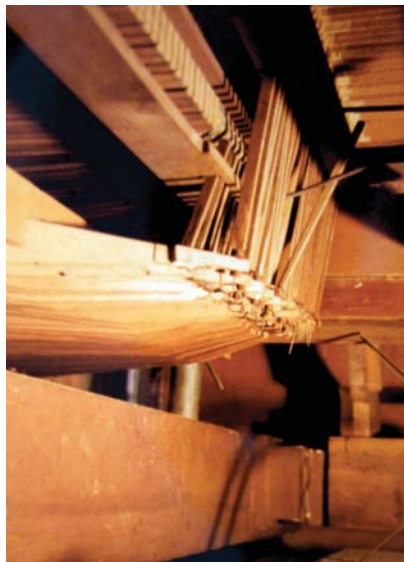
The back of the angled backfalls from the pedal coupler, showing the stickers to the tails of both manual keyboards. The stickers are carried in boards that move laterally to engage the stickers under the key tails. Note the sticker which has fallen out of its guide slot.
