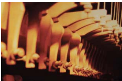
These squares have tapped wires, felts, and leather buttons for adjustment.
