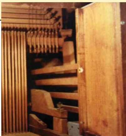
A view from the console showing the back of the Swell keys at bottom, the stickers from the Great extending upward through the Swell key tails, and the Great rollers at the top that activate the diatonic bass notes. The rollers and squares at the top right activate the Great pallets d#, c#, B, A, G, F, D#, C#. The Great pallets C, D, E, F#, G#, A#, c, d, e, f . . . g''' are activated from left to right by the fanned squares.
