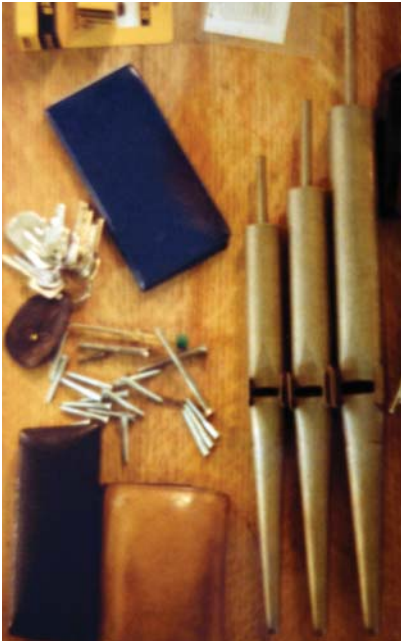
Pipes from the 4' Flute à Cheminée. These pipes were constructed in the classical manner with planed common metal, soldered and domed tops, chimneys with no tuning devices, and very large ears for tuning. These pipes are shown with the ears in a normal position.
