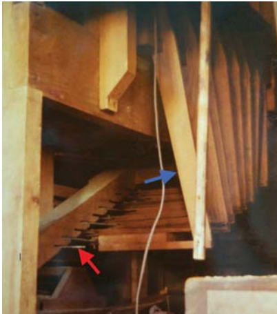
The red arrow points to the metal squares to which the Great stop knob shanks are connected. The horizontal shanks connected to those squares activate the large, vertical backfalls indicated by the blue arrow, which in turn activate the ends of the sliders on the Great windchest.
