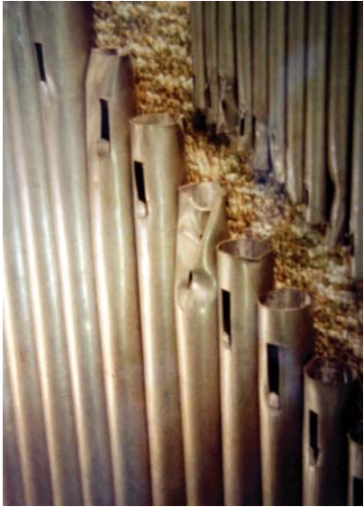
The 8' Keraulophon prior to restoration, showing the crudely pinched tops of the pipes to effect a pitch reduction.
