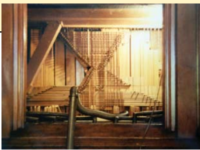
A view above the console with the façade center flat pipes removed. The Great windchest is at bottom with zinc wind conductors to the façade pipes. The Swell rollerboard is above and behind the Great windchest. The treble pipes of the Pedal Double Open Diapason can be seen to the left of and behind the Swell rollerboard. The wind trunk to the Swell windchest can be seen at upper left, extending diagonally. The Swell windchest now extends above the Great windchest, encroaching upon the clearance of the tallest pipes on the Great windchest. The large black vertical tube is part of a vacuum cleaner.
