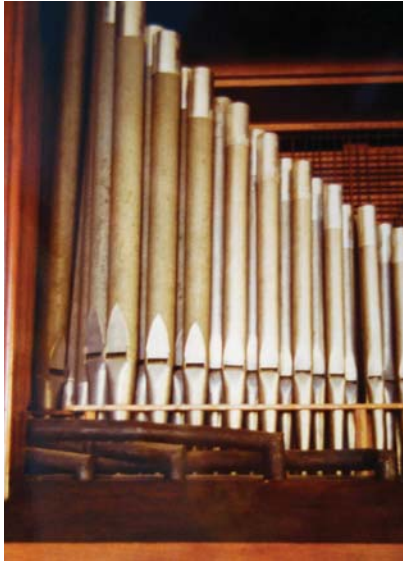
The Open Diapason on the chest. Note the planed metal feet and zinc resonators of the tenor pipes. Tuning slides were added during the restoration.
