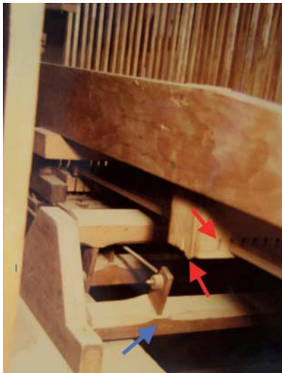
View from the back, looking towards the rear of the keyboards. The blue arrow points to one of the axles from one of the couplers that activates a movable board with the stickers. The red arrows point to a guide rail for the Swell trackers; note the crudely cut end of the rail and the guide missing a tracker run. This may be the result of the repositioning of the Swell chest in the Piru installation.
