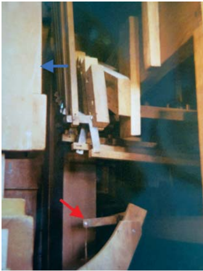
The squares and shanks of the stop action to the Swell windchest from the left stop jamb. The blue arrow points to a pipe of the Pedal Double Open Diapason; the red arrow points to the vent valve for that stop.
