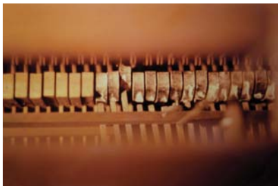
The tails of the Swell keys, showing rounded and leathered ends where the pedal coupler stickers engage them. Note the wear on the leather. Also note that the stickers lean to the left, which is caused by a misalignment in the pivots of the angled pedal backfalls, a casualty of wear and the installation of the balanced swell pedal.
