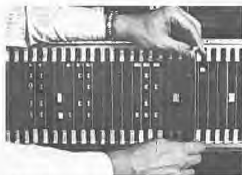
All tone generation is contained within the console. Separate plug-in circuit boards provide selective control over the timbre, tuning, and articulation of individual stops.
