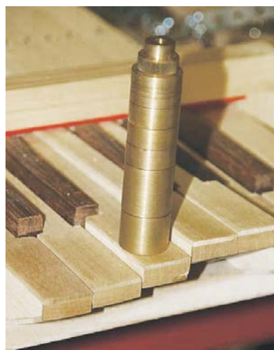
Figure 2. Flexibility in the action just before the pluck point demonstrated by placing a 200g key weight on the key head. Model organ, University of Edinburgh
