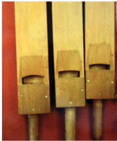
Stopped pipes from the bass C to F# of the Swell 8' Open Diapason. Note the lightly arched mouths.
