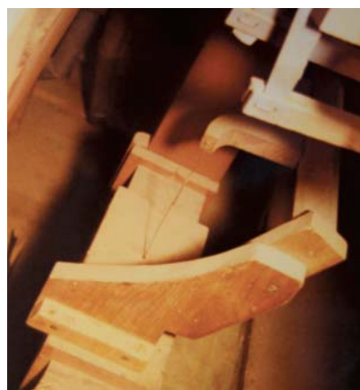
The stopknob of the Pedal Double Open Diapason is connected to a ventil which feeds all three windchests of that stop. The wire is connected to a valve in the wind trunk. The wire is activated by the wooden trundle, which is itself connected to the stop knob at the console.
