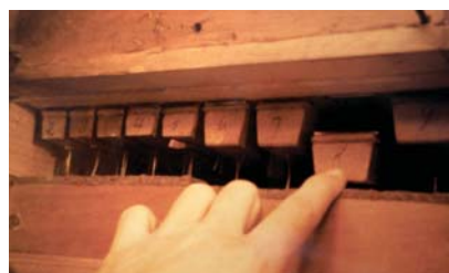
The C-side Pedal chest showing the arrangement of the pallets. The low D pallet is held open.
