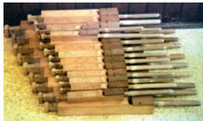
Stopped pipes from the Swell 16' Bourdon that were placed on the chest.
