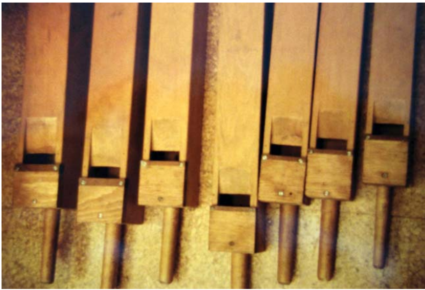
Open pipes from bass G to tenor E of the Swell 8' Open Diapason. Note the virtually identical mouth heights (cutups) of these pipes with no arching.
