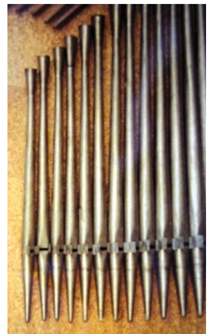
8' Viole d'Amour pipes which show their construction as a Bell Gamba.
