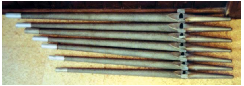
Bass pipes from the Swell 4' Principal have tapered zinc resonators and very high, arched mouths.
