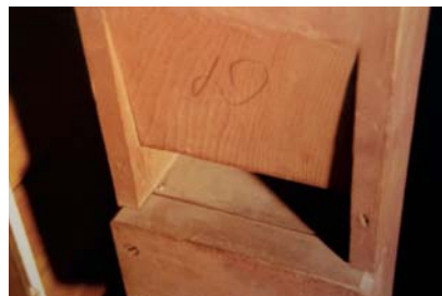
The mouth of the low D of the Pedal Double Open Diapason. Note the absence of beards, rollers, arching of the mouth, and nicking. This is a classically-constructed pipe with superb blend and a powerful, tactile effect.
