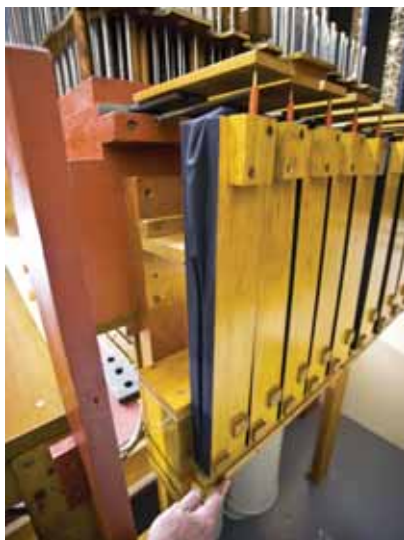
Rebuilt Swell slider mechanisms in the Newburyport organ
