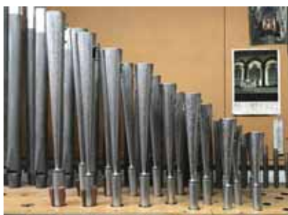
The pipes of the Choir-Solo 8' French Horn during pre-voicing in the Létourneau workshops
