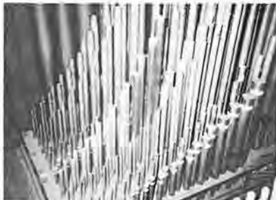
Restored pipework in Grand Orgue division.
