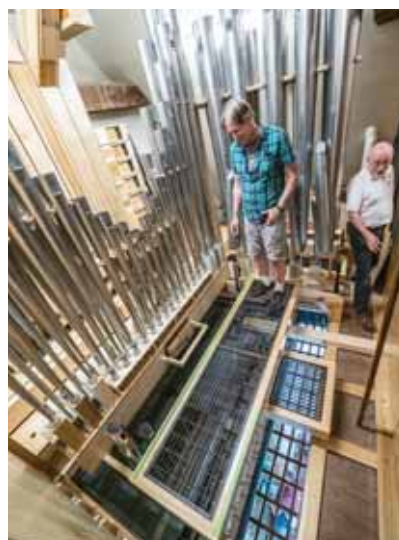
Organ technician David Storey, a Dobson alumnus and Opus 96's curator, inspects the organ during voicing. Seen here are Pedal pipes and walkboards built with grilles to permit passage of sound down into the church. (photo credit: Wm. T. Van Pelt)
