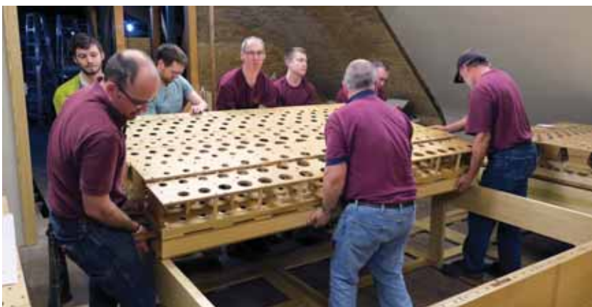
Installation of one of the three Swell slider windchests (photo credit: Lynn A. Dobson)
