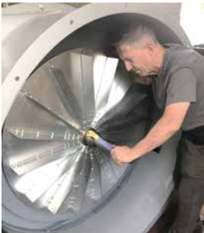
Joe Sloane installing new fans in a large organ blower (photo credit: Steve Dickinson)
