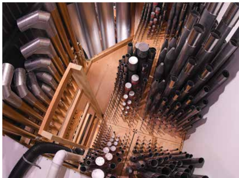
The Great division, with its pipework arranged in major thirds, is high in the casework, close to the central axis of the church.
