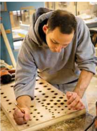
Quality control—ensuring that counter-sinking is correct: Anthony Peragallo notating the burn marks on the top of a windchest. Pipes sit in the depressions on the top of the windchest.
