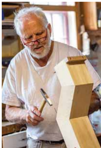
A mitered air trunk. After applying glue to the joints, finishing nails are used to hold the pieces in place. (Moore)
