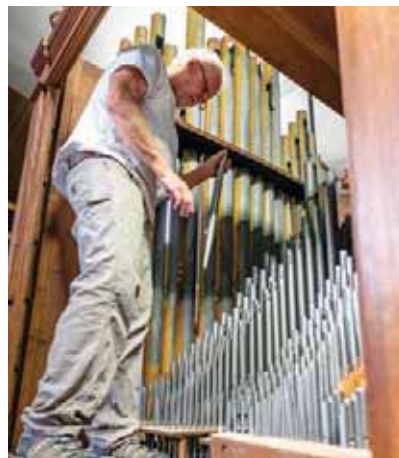
Tuning the Hook & Hastings in the erecting room. This is a stock model two-manual instrument dating from around 1910. (Moore)
