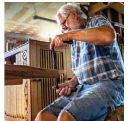
Rounding the end of a wooden reed pipe using a draw shave (Moore)
