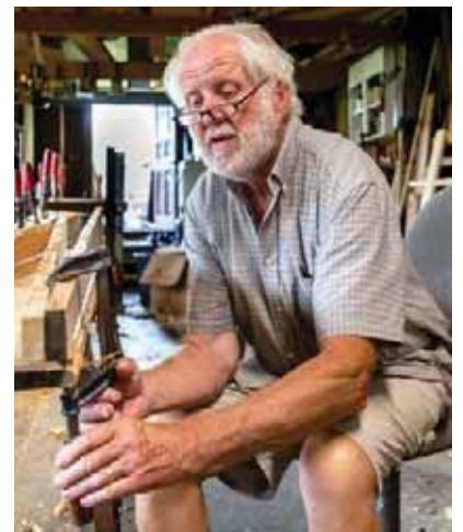
David Moore clamping up a 16' Trombone, a wood reed stop. This is a replica of a stop in an E. & G. G. Hook organ.
