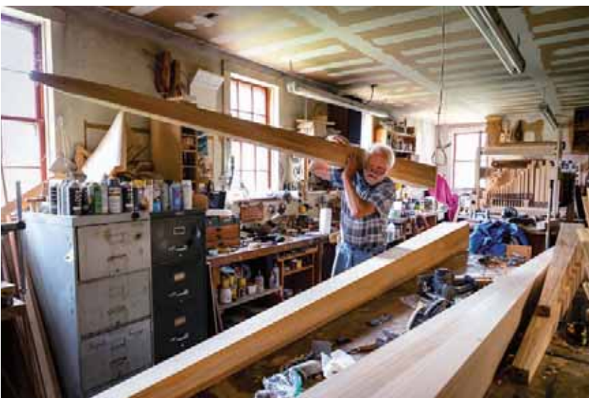
Carrying one of the 16' Trombone pipes from wood shop to erecting room (Moore)
