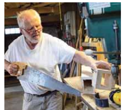
Cutting an air trunk. The chop saw was able to get through about 90% of the windtrunk. The job is finished with a handsaw. (Moore)
