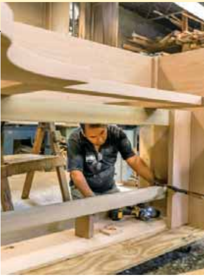
Setting the expression shoe bar in a console under construction (Peragallo)
