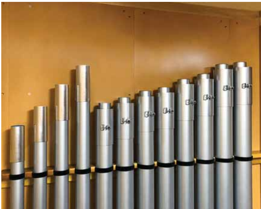
Great 8' Corno Dolce pipes employ Haskell tubes from G down to reduce height
