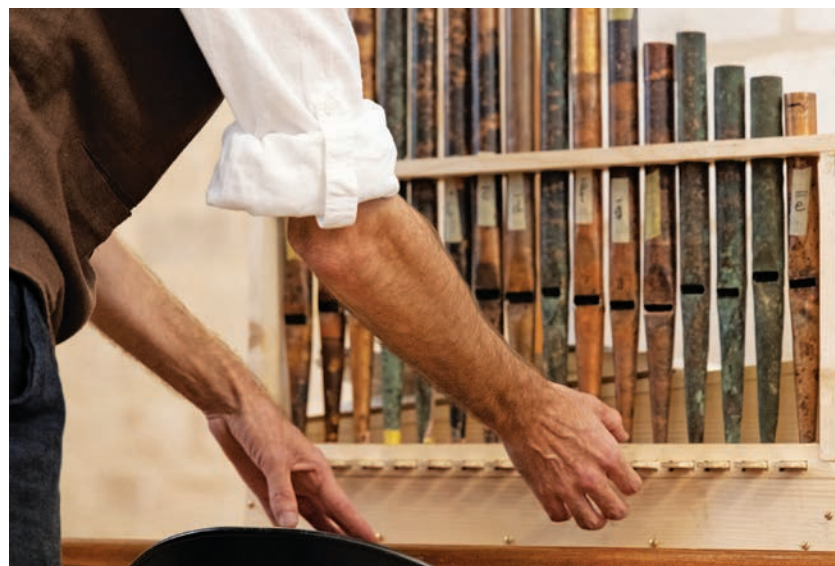
David Catalunya demonstrates the slides opening and closing the wind for each pipe
