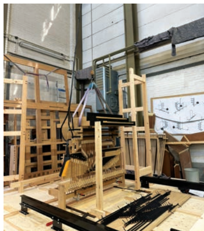
Beginning of erecting organ for Japan. The black steel is the frame that connects Rugwerk with the main organ case. The keyboards are suspended from the ceiling temporarily. (photo credit: John Bishop)
