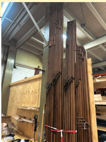
Rollerboards from Schniger organ in Zwolle (photo credit: John Bishop)
