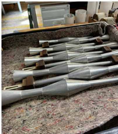
Viool da Gamba in process for restoration of Schnitger organ in Zwolle, copied from Schnitger in Alkmaar. Photo shows resonators only. (photo credit: John Bishop)
