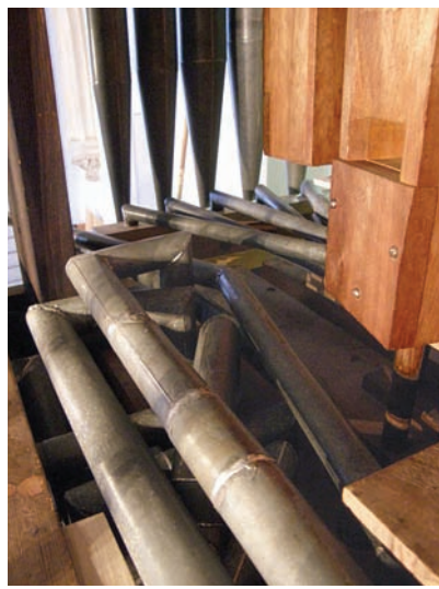
The zinc tubing must be accurately re-paired if it is to fit
