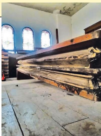
Large double-rise reservoir ready to be releathered (photo credit: Brian Sprague)
