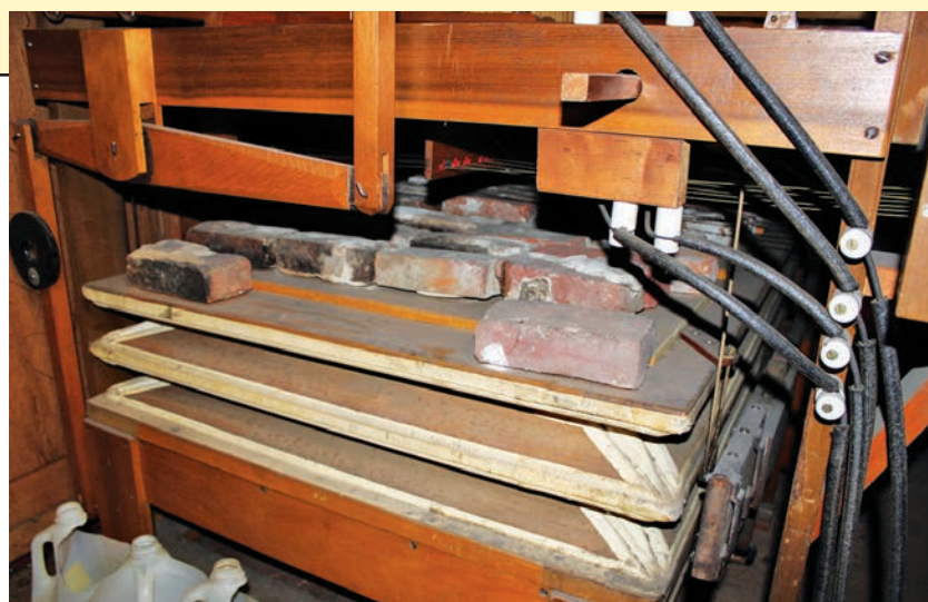
Large double-rise reservoir ready to be releathered (photo credit: Nick Wallace)
