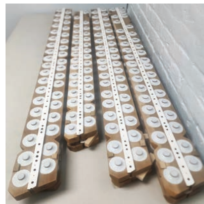
Note pouches of a pitman windchest (photo credit: Larry Pruett)
