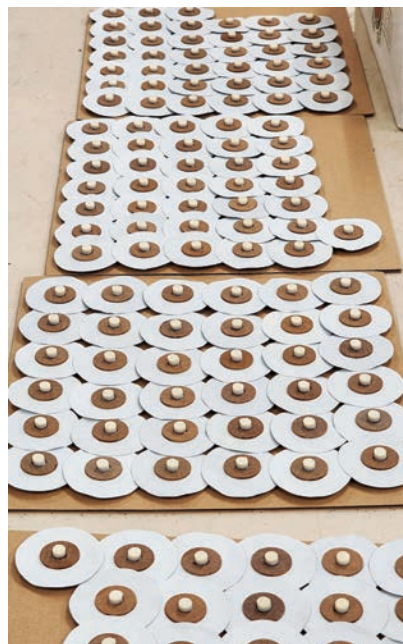
Note pouches ready to be glued on pitman rails in windchest (photo credit: Larry Pruett)
