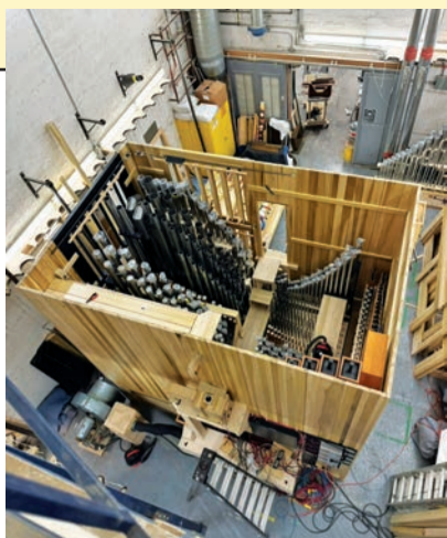
Létourneau, the Swell division for Marvin Methodist Church, Tyler, Texas. The wood structure in the back left of the box is a two-stage Swell-within-a-Swell for 8' Vox Humana. 16' Contra Fagotto is behind the shutters; an 8' Trumpet is standing on the floor in upper right corner; 16' Bourdon in the back corner of the Swell box. (photo credit: John Bishop)
