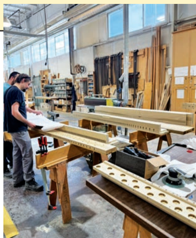
Windchest construction at Casavant (photo credit: John Bishop)
