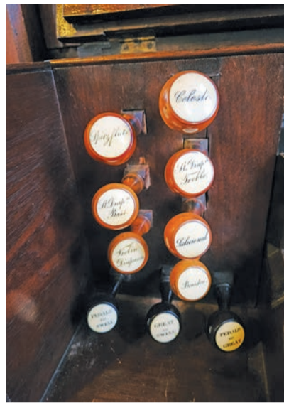
Left stopjamb showing newer Pedal coupler drawknobs (photo credit: J. A. Hefner)
