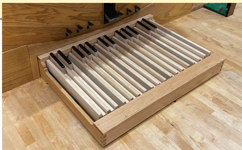
New concave, straight pedalboard with radiused sharps (photo credit: Tim Buchman)
