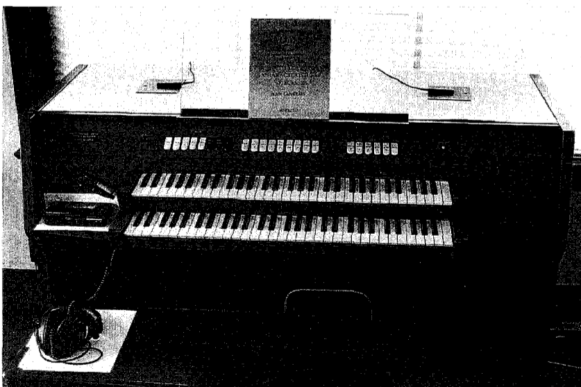
Fig. 14: Another quick and easy microphone setup using PZMs placed on top of the console. This could be ideal for situations where the organ chambers are to the left and right of the console, or in a gallery where the console is in front of the organ. Note the Walkman cassette recorder to the left of the keys.
