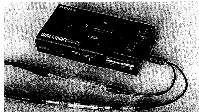
Fig. 5: The wrong way to do what is shown in Fig. 4. The numerous bits and pieces available in the neighborhood electronics store look like they should work, but multiple adapters plugged together almost invariably cause a buzz or hum.
