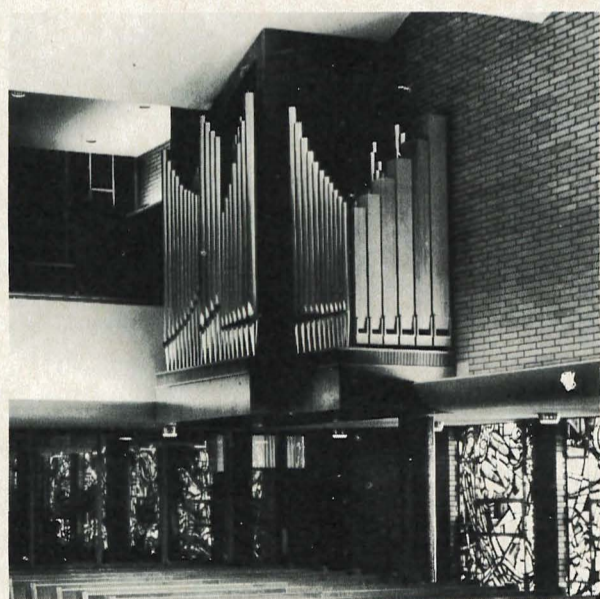
THIS ENCASED organ of 22 ranks is equipped with slider chests.
