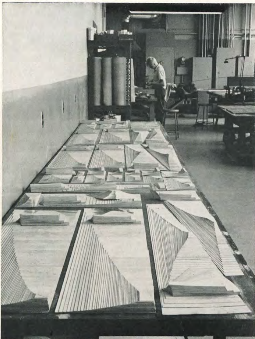
Metal for pipes cut to size for bodies and feet, ready for rounding and hand soldering. Each stack represents parts for one rank of pipes.
