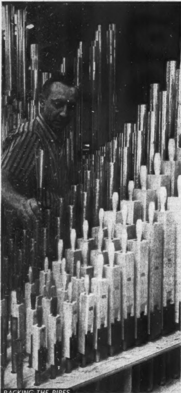
RACKING THE PIPES
