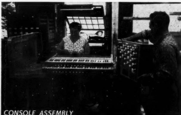
As Mrs. Adele Buehkofer solders wires of console harness to a keyboard, Paul Plog attaches a side jam containing stop controls that organist manipulates in selection of different tone colors. These include the sounds of such instruments as clarinet, trombone, harp, and bells.
