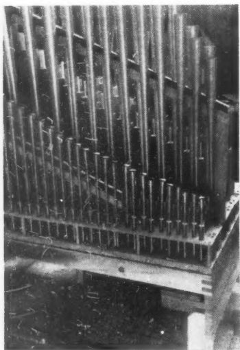
FRONT VIEW of a new pedal chest which was added to a rebuilt tracker organ. Stopped is: subbass 16 ft., principal 8 ft., pommer 8 ft., choralbass 4 ft., gedeckt 4 ft., mixture 3 ranks, fagot 16 ft., schalmel 4 ft. Pipes on this chest are arranged chromatically.
