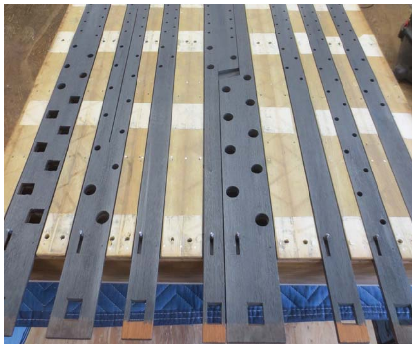
Wood sliders with steel guide pins—10,000 bangs and they're gone. (photo credit: Nick Wallace, David E. Wallace & Co., LLC)
