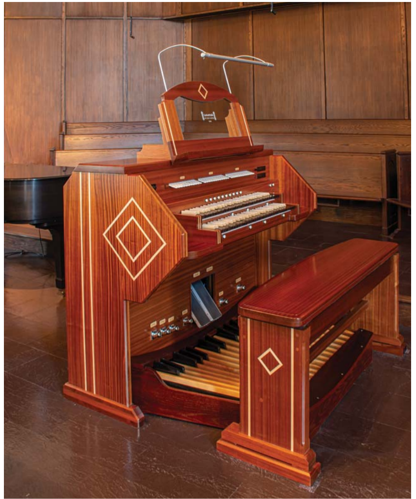
The façade as well as the new console was built from Sapele, an exotic African wood species characterized by its striking ribbon-like grain pattern.
