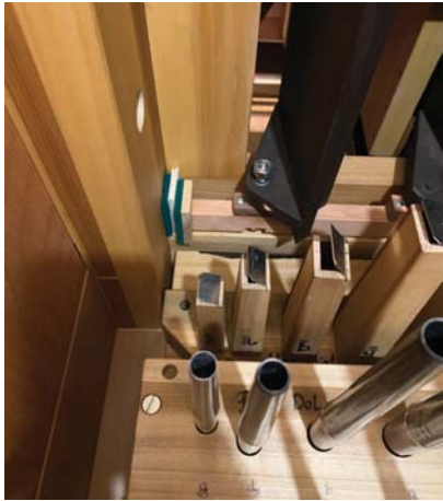
The Positive swell shade mechanism and the treble of the Hohlflöte 8' based on Schnitger models
