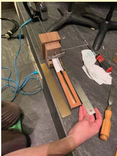
32' Posaune low C shallot, tongue, and block
