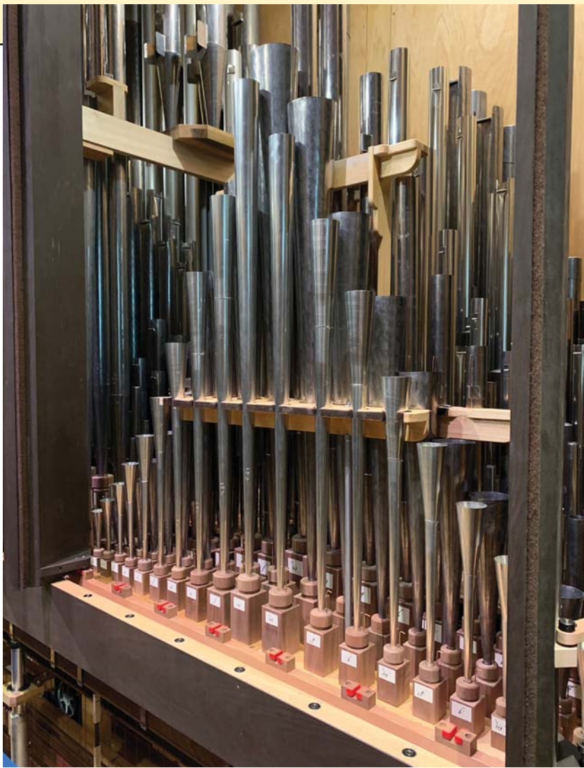
View inside the Swell division with the shades removed. The Oboe 8' is in the foreground.
