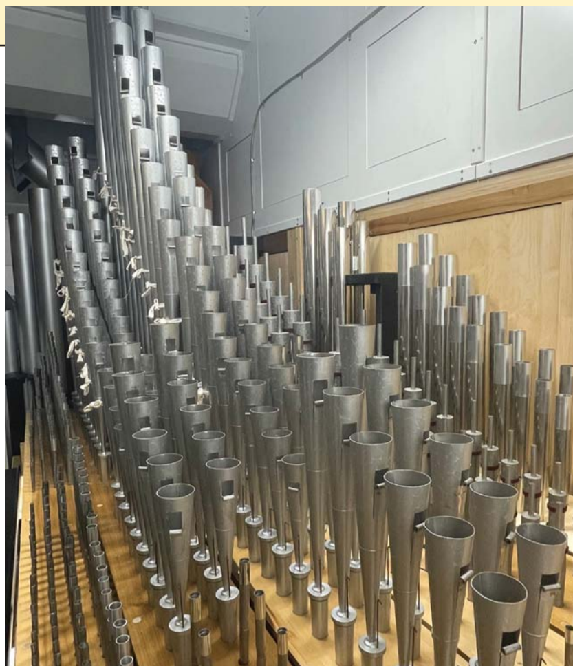
The upper Great chest, with the Mixture V, the 4' Clarion and 8' Trumpet in the foreground
