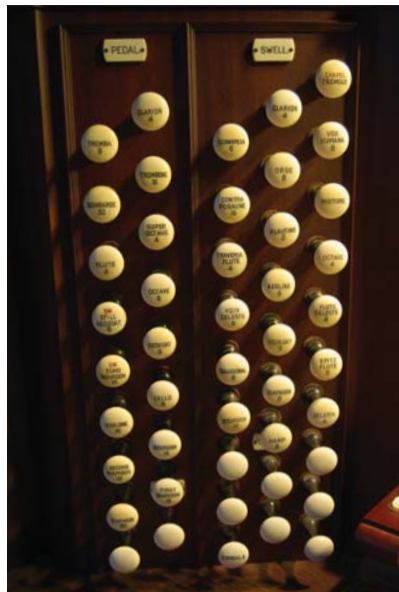
The left stopjamb of the console, featuring the Swell and Pedal divisions
