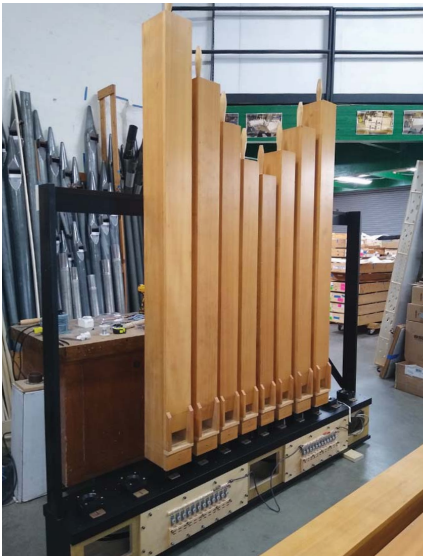
The Swell Lieblich Gedeckt offset chest for the bottom octave is being assembled and pipes racked in the shop.
