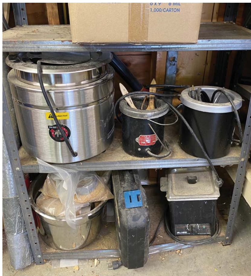
Hot pot, glue pots, ultrasonic cleaner (photo credit: John Bishop)
