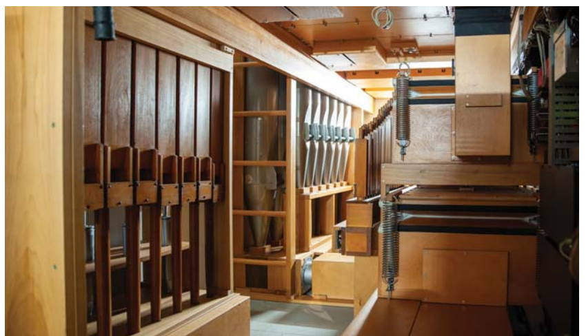
Pedal pipework and wind reservoir
