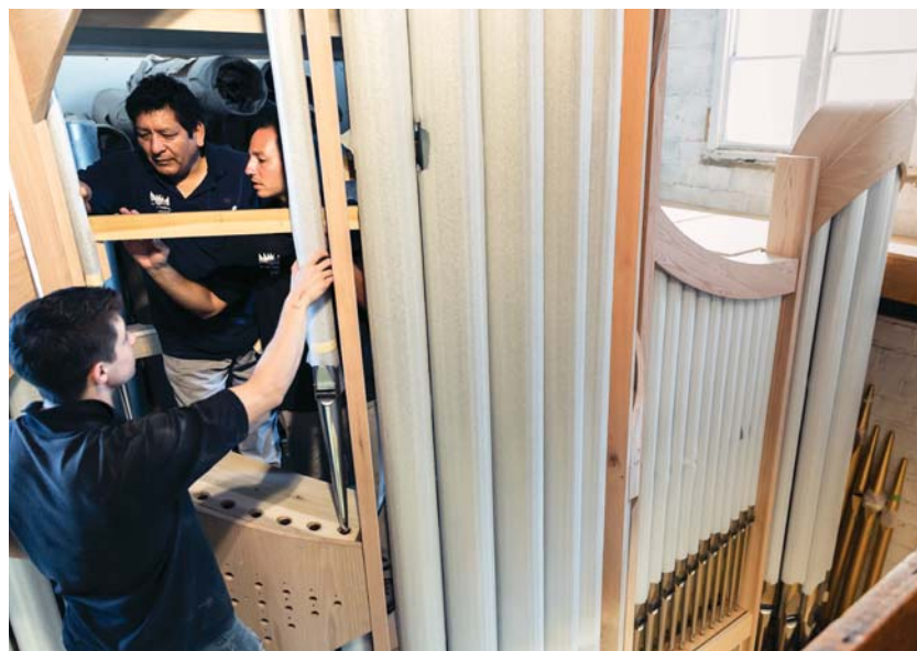
Installing façade pipes. The instrument, built for the Cathedral of Saints Simon and Jude in Phoenix, Arizona, is in the Peragallo erecting room.
