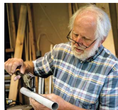
Soldering the seam on a metal pipe. With the exception of the seam area, the pipe is coated with “size”—a mixture of ground calcium carbonate and gum arabic. The solder does not adhere where the pipe is coated with size. (Moore)
