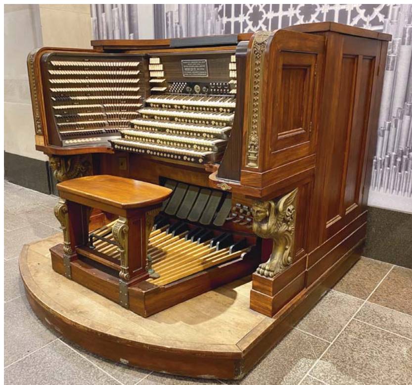
A second, “portable” console is currently on display in the lobby of Boardwalk Hall. It was connected by a multi-core cable measuring 150 feet and has five manuals and 673 stopkeys.
