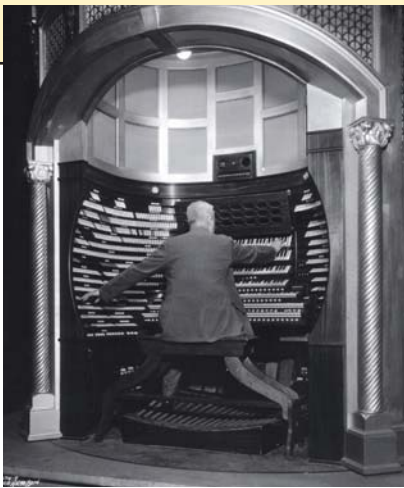
Emerson Richards demonstrates the ergonomic design of the console by reaching for the furthest keys of the uppermost manual while manipulating the outermost stop-keys on the opposite side.
