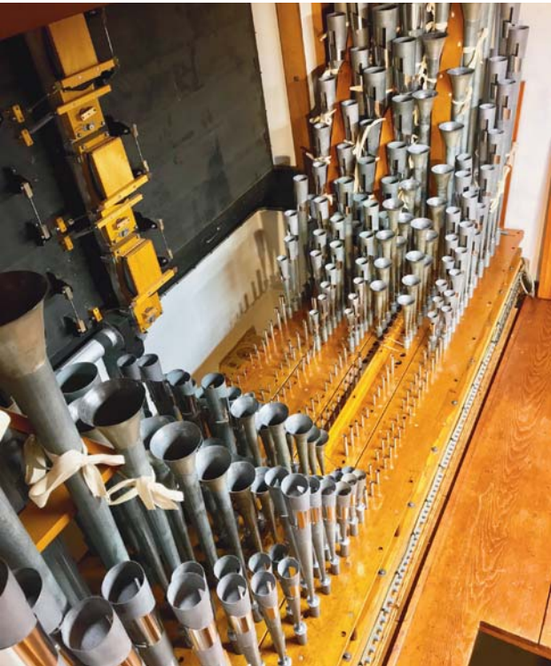
The Swell high-pressure (30'') reed chorus. From left to right: Double Trumpet 16', Harmonic Trumpet 8', Field Trumpet 8', Harmonic Clarion 4'
