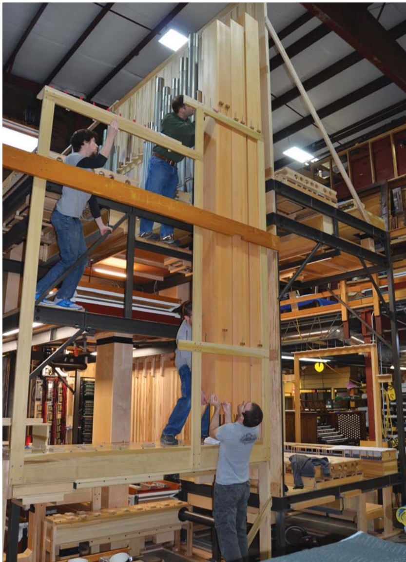
Crew installing pedal pipes in Parsons' workshop
