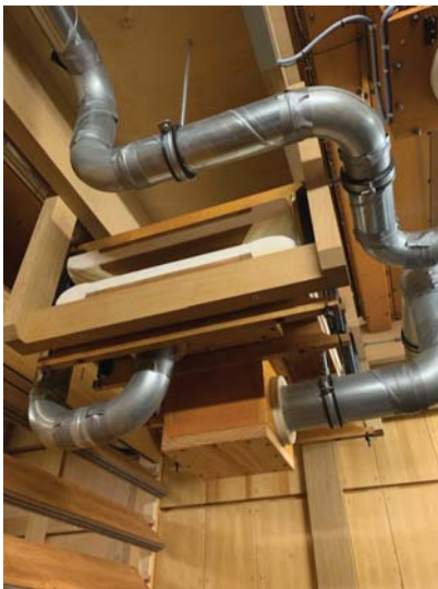
A Skinner regulator with metal windlines. The regulating cone valve is in the box on the bottom. Evangelischer Saalkirche, Ingelheim am Rhein, Germany (the only Skinner organ in Germany). (photo credit: John Bishop)
