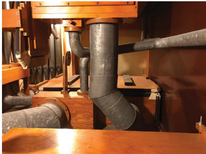
In this Aeolian-Skinner organ, the pulley on the stand is mounted on the curtain valve, which is connected to the top of the regulator with a braided string. (photo credit: John Bishop)
