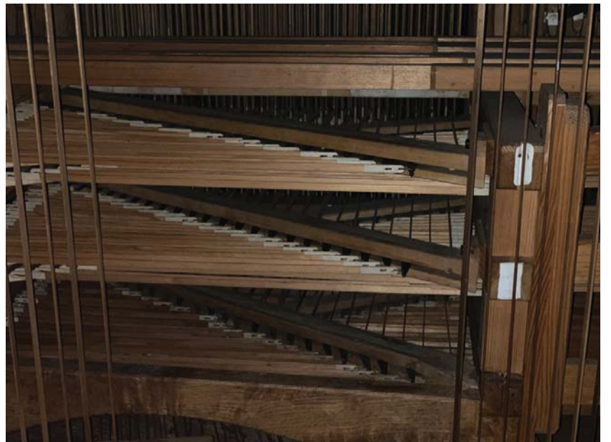
Tracker keyboard action under a four-manual console, 1750 Gabler organ, Weingarten, Germany. (photo credit: John Bishop)
