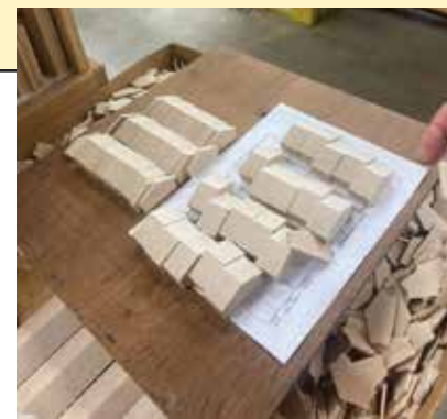
Coupler rail dividers at Organ Supply Industries. They remind me of houses and hotels in "Monopoly." (photo credit: John Bishop)
