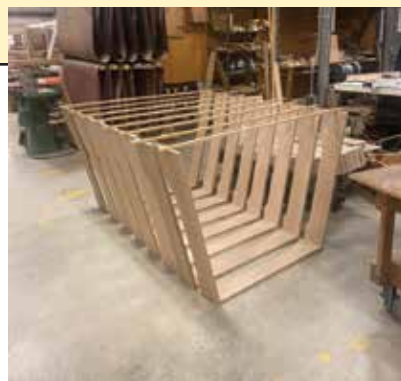
Eight pedalboards in production at Organ Supply Industries; large sanding belts hanging on a rack behind (photo credit: John Bishop)
