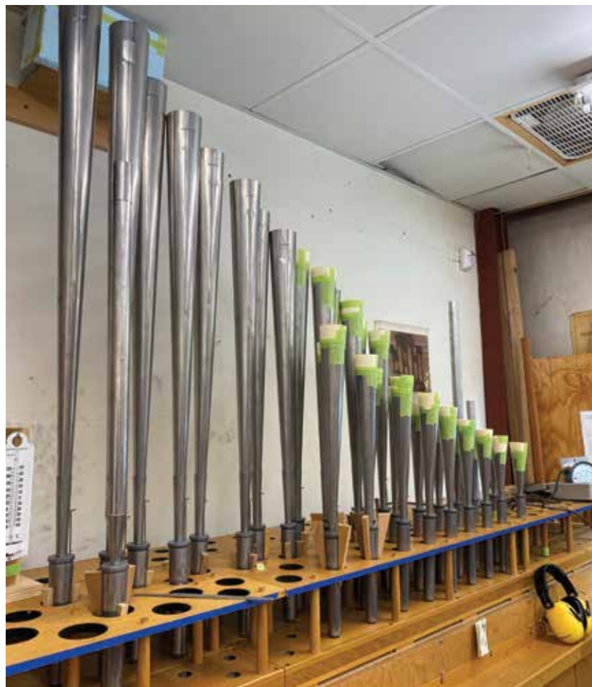
Great 8' Trompette with extender templates on voicing jack at C. B. Fisk (photo credit: Jared R. Stahler)
