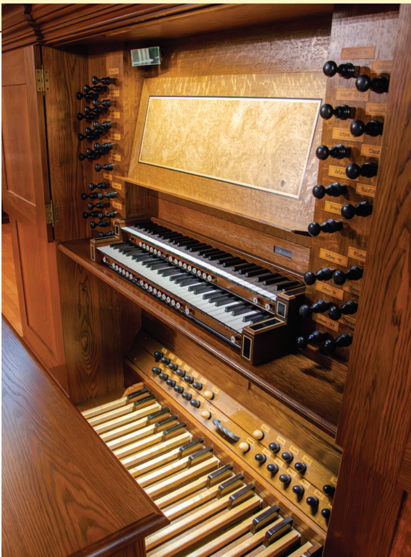
Keydesk, with burl oak veneered music rack and hand-lettered stop labels on leather
