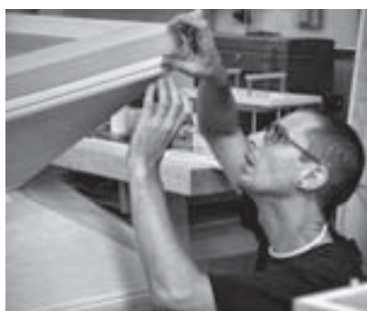
Dean Ekmann applies corner reinforcement gussets to the wedge bellows
