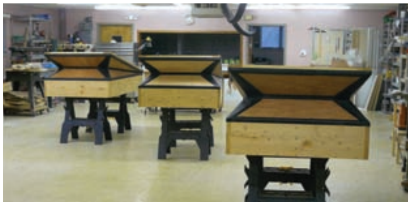
Three wedge bellows provide wind to the organ, one for each division (pictured in the shop)
