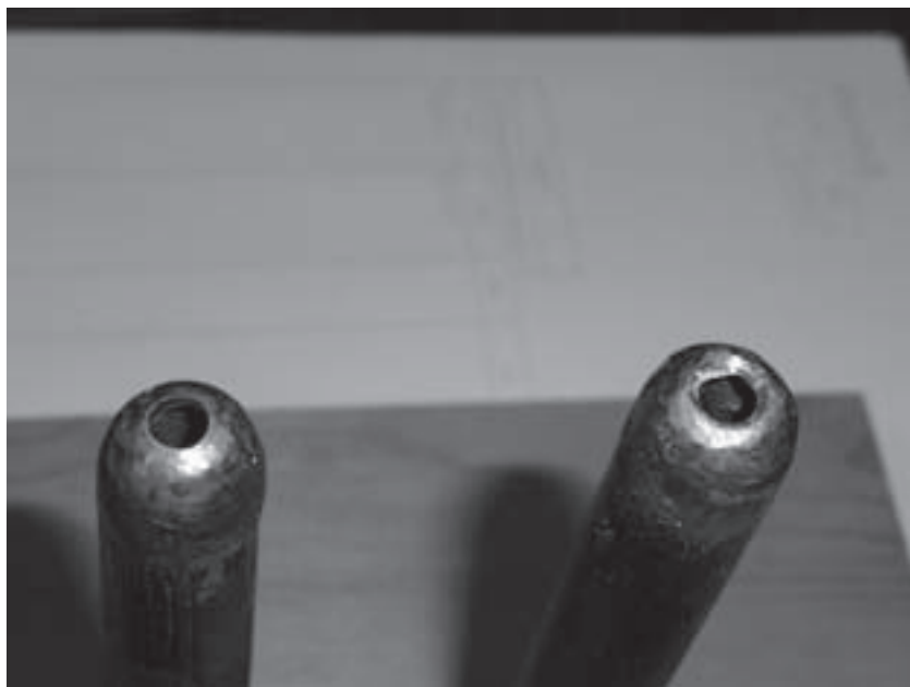
Photo 1. A noisy toe and a quiet toe. The toe-hole on the left has a short straight section that creates noise when air passes through it. The toe-hole on the right has been countersunk to eliminate the noise.
