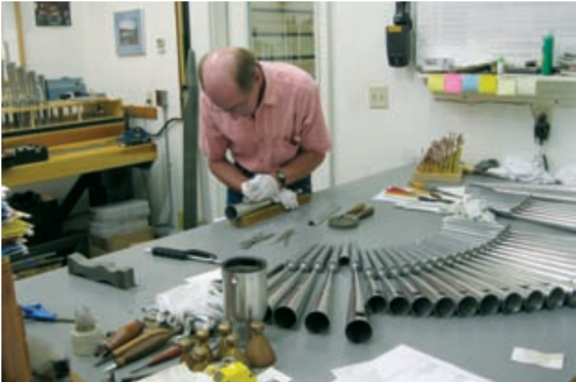
Eric Johnson in the process of cutting the flaps on the Swell unit Trumpet
