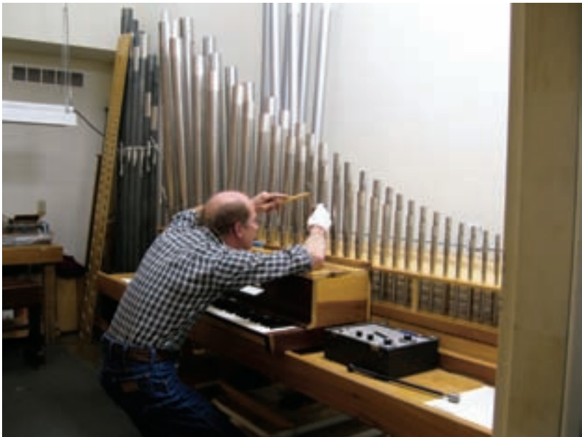
Eric Johnson in the process of voicing the Swell 4' Principal
