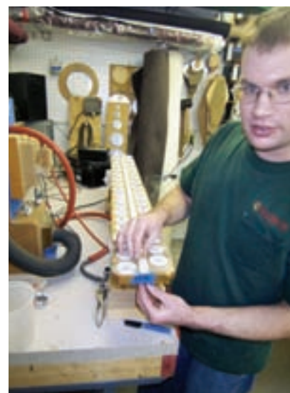
FBI tech Adam Lagocki shop tests one of the organ's many pouch rails.
