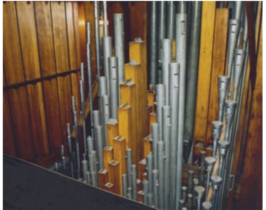
8' Orchestral Oboe, 8' Clarinet, 8' Voix Celeste (flared), 8' Concert Flute, 4' Flauto Traverso, 8' Gamba (flared), 8' Vox Humana, and 8' English Horn
