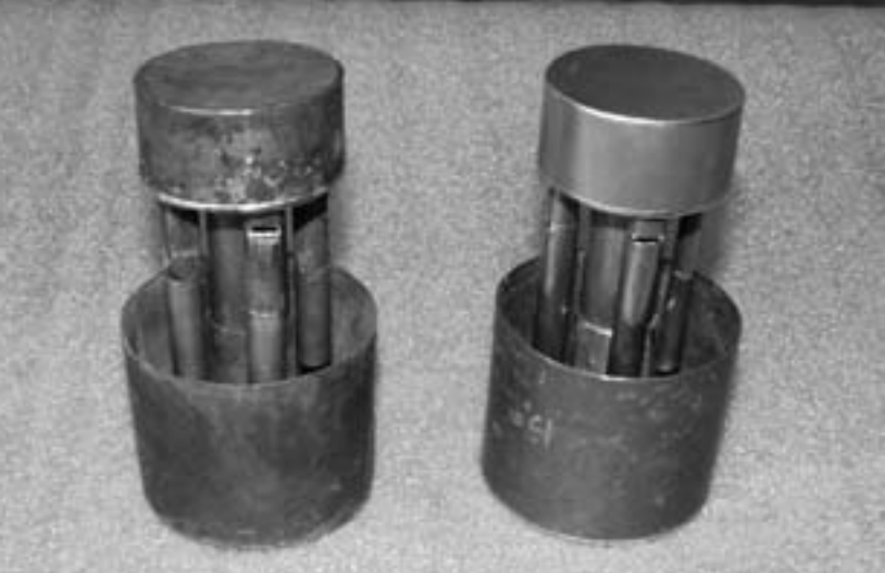
Photo 4. The two Uccelliere (Nightingales) in the Venafrò organ. Their round shape is rare and unusual. The one on the left is original. A second, identical unit (right) was missing, and had to be rebuilt during the restoration of the instrument.
