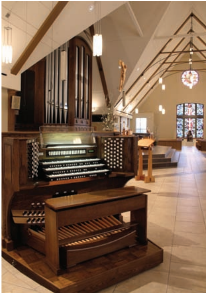
Console on movable platform (photo credit: Deana Graham)
