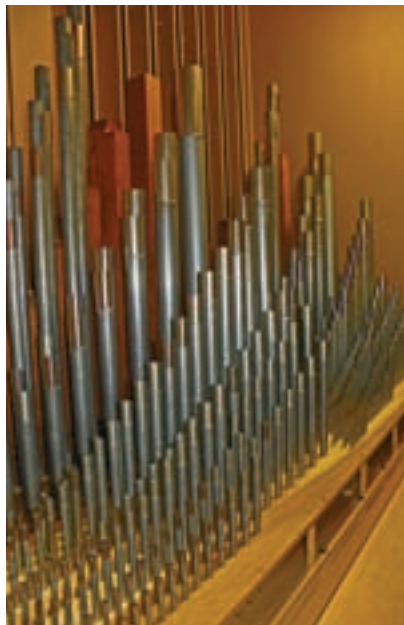
The main slider soundboard in the Swell department, arranged in a "saw tooth" whole-tone layout (photo: Sebastian M. Glück)
