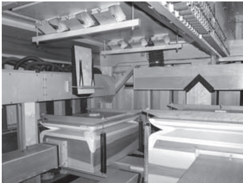
Hayes Barton organ Opus 39 winding system under Swell
